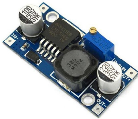
Figure 5. Description of LM2596M module.
