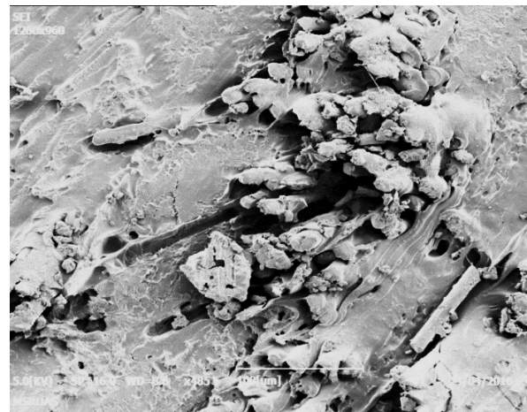
Figure 21. Drilled hole surface of the B.C. without support post tool wear.
