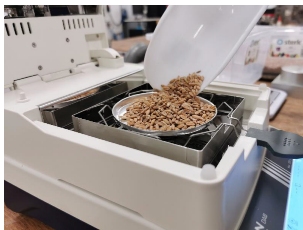
Figure 4. Moisture content meter
