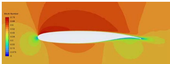
Figure 11. Mach number contour around NASA sc (2) 0712 at AOA 0° - 3D case
