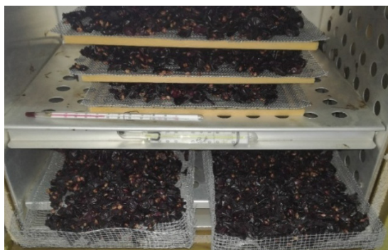
Figure 1. Oven drying of grape pulp at 40°C
