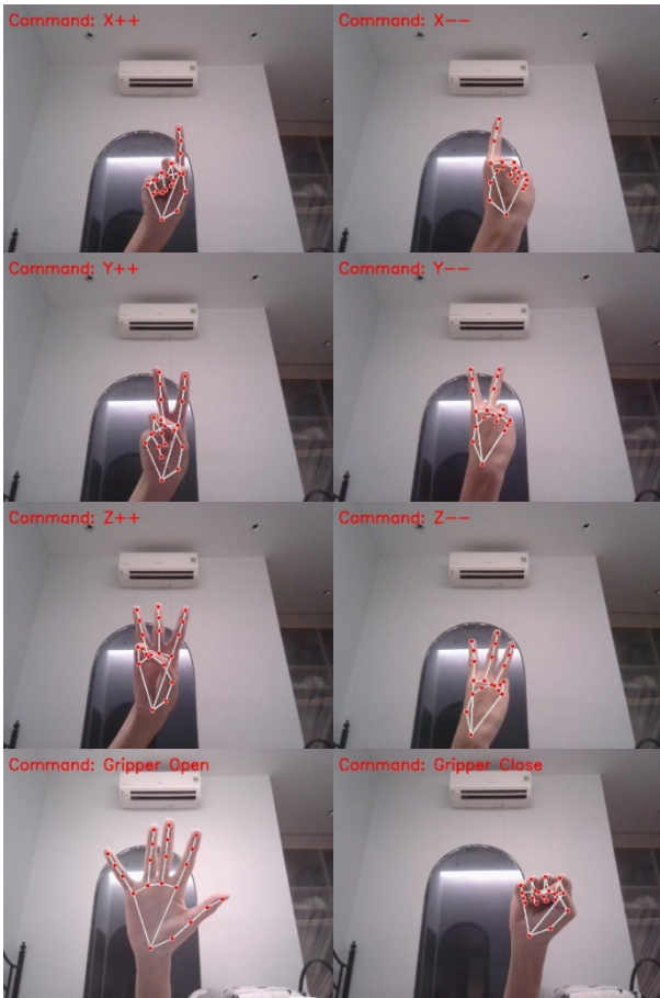
Figure 19. Hand gesture recognition results mapped to robot control commands.
