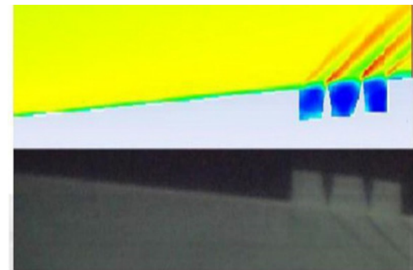
Figure 12. Comparison of the Numerical and the experimental shock structure for STD
