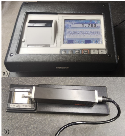
Figure 4. Surface roughness tester, a) Display unit, b) Detector unit
