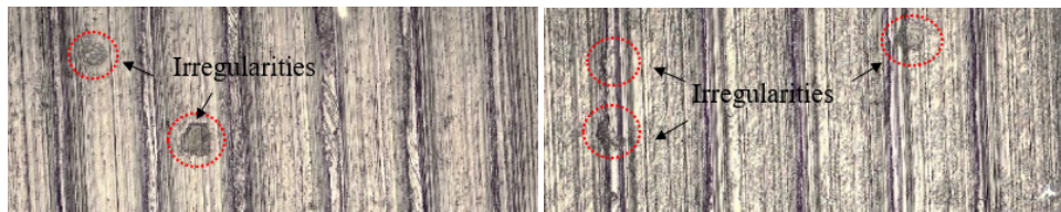
Figure 12. Machined surface texture observed by optical microscope Eclipse LV150N Nikon at X10 magnification
