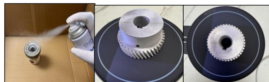
Figure 3. Application of 3D scanning spray on the helical gear
