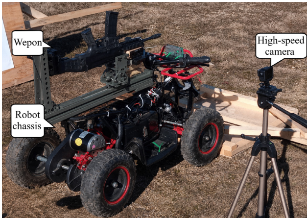
Figure 14. Experimental measurement of robot vibrations.
