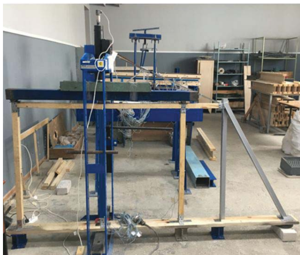
Figure 5: Scheme (a) and general view of experiment (b) for frame specimen: 1 – distributive; 2 – frame legs; 3 – girder; 4 – support beam
