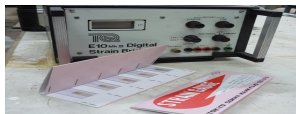
Figure 4: Electrical resistance strain gage and strain gage indicator
