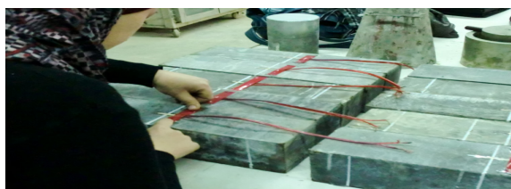
Figure 3: Electrical resistance strain gage attached at the mid-section of the specimen
