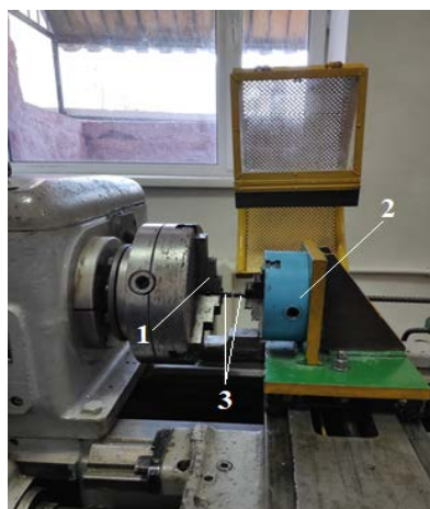
1 – three-jawed lathe chuck; 2 – three-jawed special device chuck; 3 – fixed workpieces
