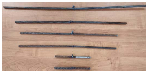
Figure 3. Some reinforcing bars joint by friction welding
