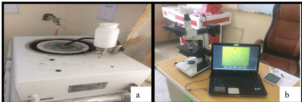
Figure 4. (a) Grinding and polishing machine, (b) Microstructure characterization device
