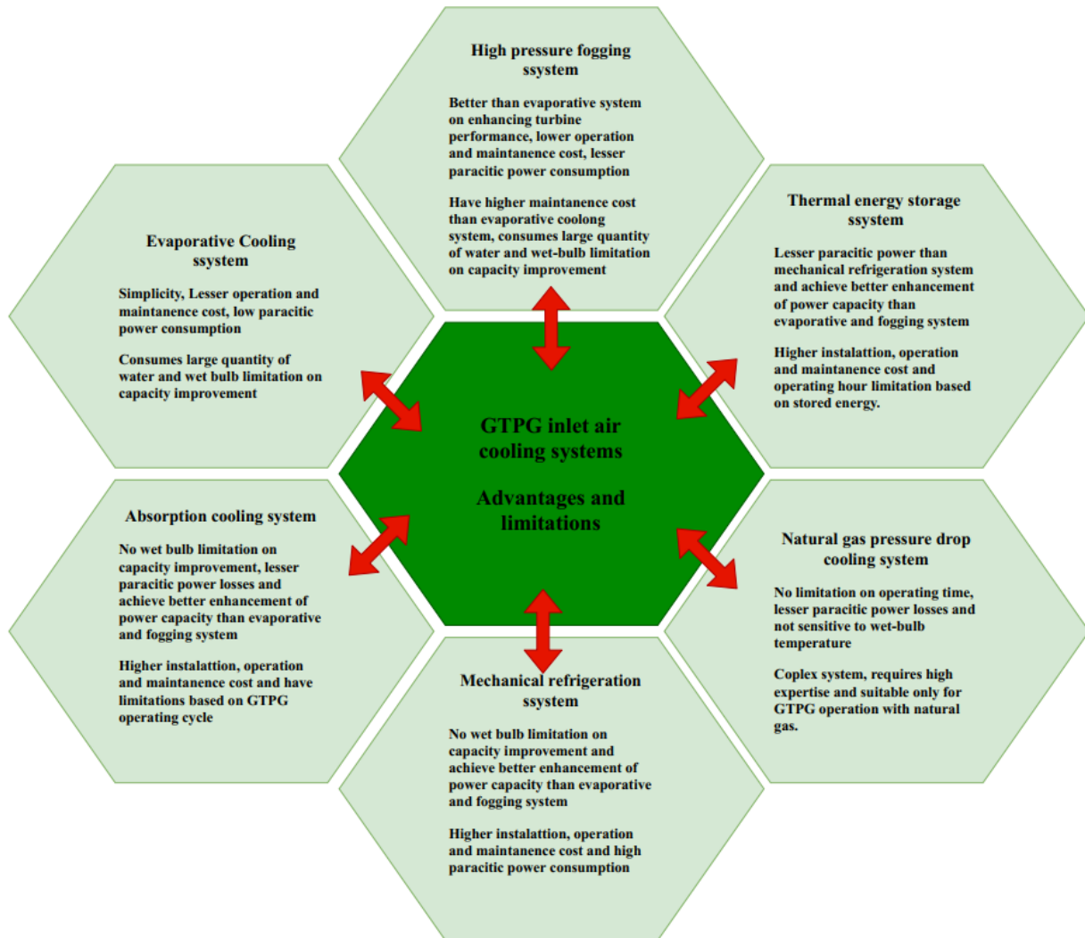
Figure 2. Comparison of different inlet air cooling methods for GTPG. Source [17]
