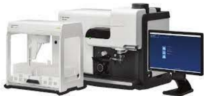
Fig.7. Agilent MP-AES 4210 apparatus for measuring the elements' mass concentration in a sample
