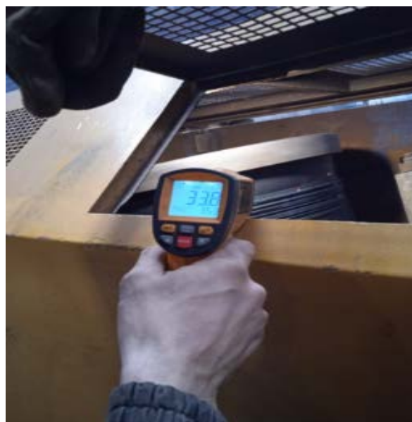
Fig. 4. Drum temperature measurement using a TK-5.04 thermometer
