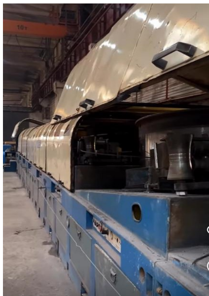
Fig.3. Kaz-Metiz LLP drawing benches (photo taken from the website of Kaz-Metiz LLP)
