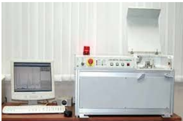
Fig.6. «SELA Matrix Continuum» apparatus for precipitation qualitative analysis
