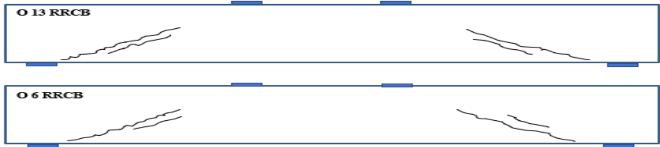
Fig. 7. Beams Failure in Terms of Crack Pattern (HRRCB &amp; SRRCB)
