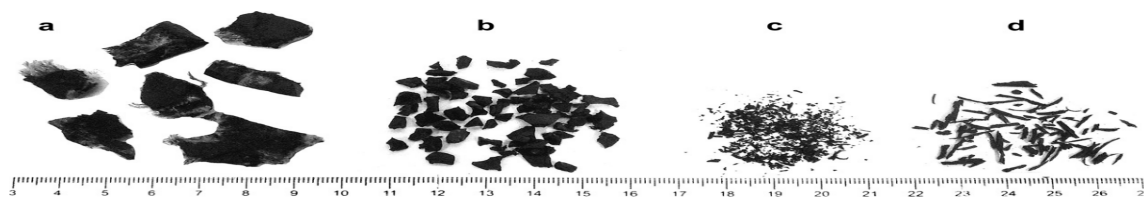
Fig. 1. Categorization of waste rubber aggregates: (a) chipped, (b) crumb, (c) granular, and (d) fiber [34]
