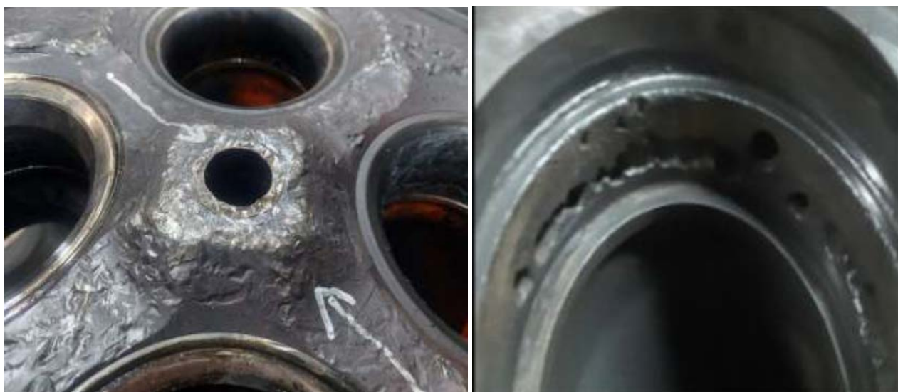
Fig. 2. of the cylinder head crack
