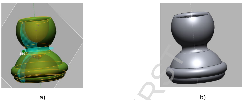
Fig. 9. (a) Application of the REVOLVE operation; (b) reconstructed 3D CAD model
