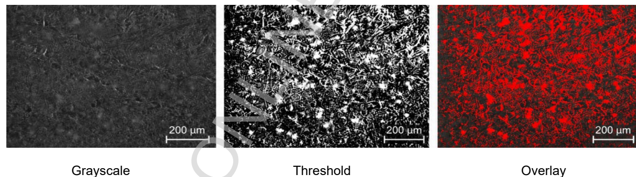
Fig. 11. Optical micrograph and ImageJ segmentation of the weld metal at a welding speed of 50 cm/min using a 50× objective lens; scale bar = 200 μm
