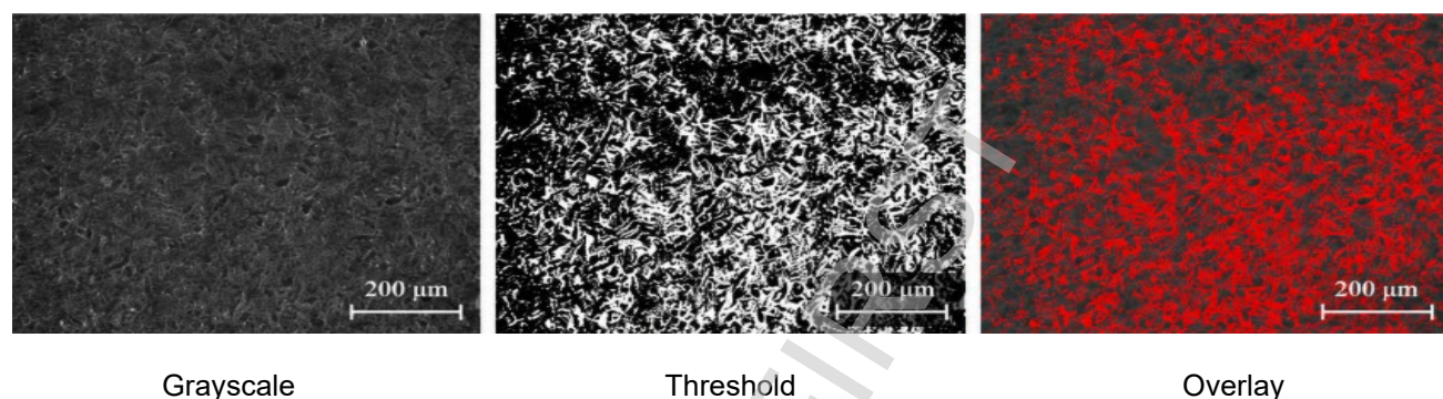
Fig. 10. Optical micrograph and ImageJ segmentation of the base metal at a welding speed of 40 cm/min using a 50× objective lens; scale bar = 200 μm
