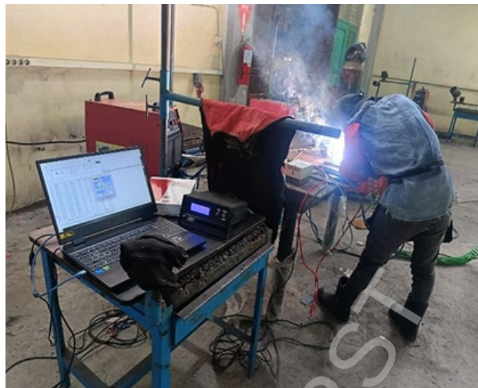
Fig. 3. Shielded metal arc welding (SMAW) process
