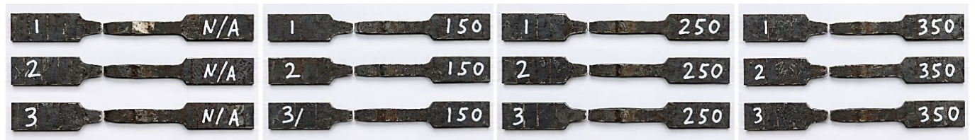
Fig. 8. Post-fracture tensile specimens under different preheating conditions
