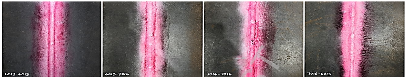
Fig. 2. Visual inspection and liquid penetrant testing results of SMAW joints with electrode combinations: (a) E6013–E6013, (b) E6013–E7016, (c) E7016–E7016, and (d) E7016–E6013
