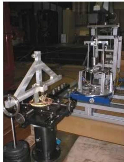
Figure 6. Calibration of the six-component external balance
