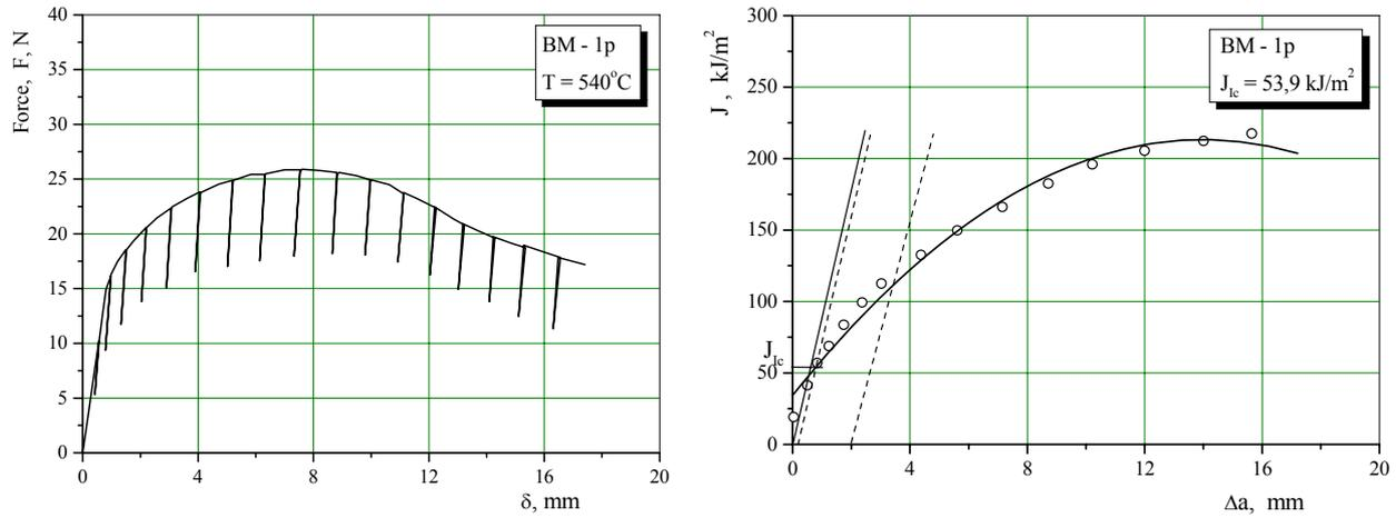
Figure 2. Diagrams  $F - \delta$  and  $J - \Delta a$  for the specimen with a notch in BM for operating temperature [9]
