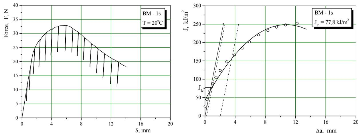
**Figure 1.** Diagrams  $F - \delta$  and  $J - \Delta a$  for the specimen with a notch in BM for room temperature [9]
