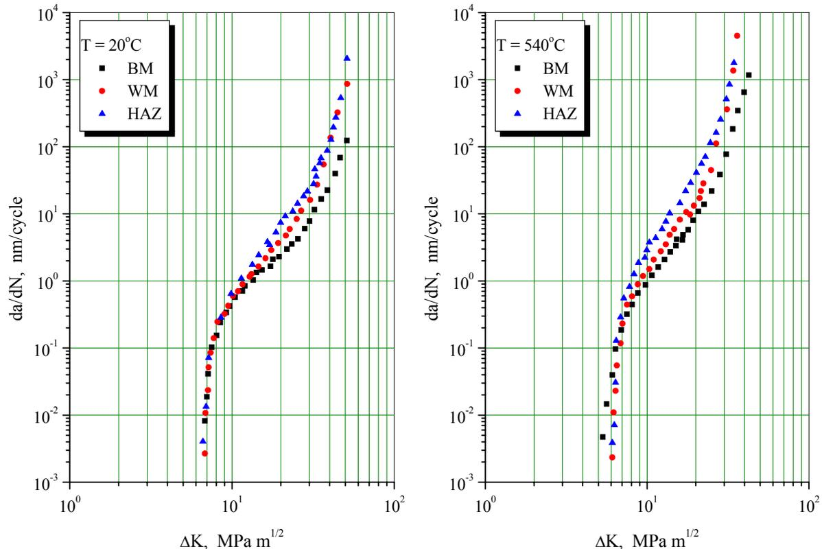
Figure 4. Fatigue-crack growth rate per cycle,  $da/dN$ , vs. The stress-intensity factor range,  $\Delta K$ , specimens pre cracked in BM, WM, and the HAZ tested at room temperature (left) and at  $540^{\circ}\text{C}$  (right) [9]
