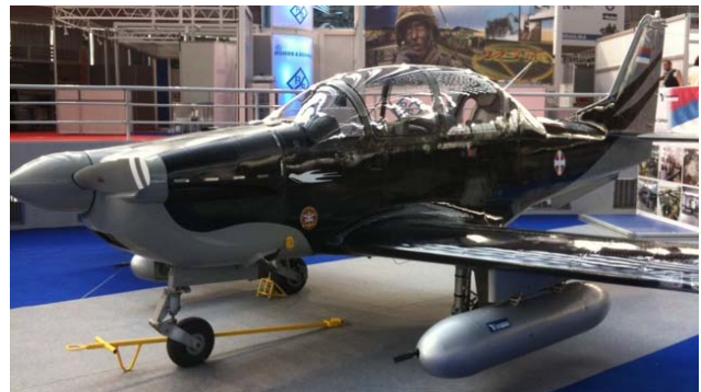
Figure 1. A 12.7mm machine gun suspension pod designed for trainer-combat aircraft LASTA (SWALLOW)
