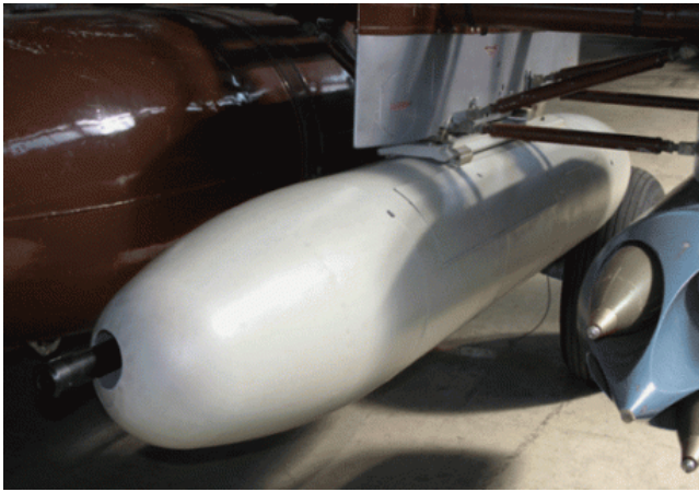
Figure 2. A 20mm automatic canon suspension pod designed for helicopter Mi-17
