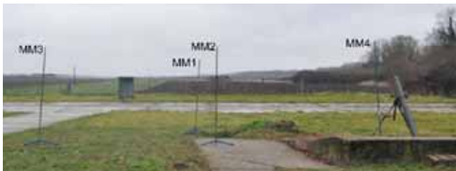
Figure 7. Display of measuring points for overpressure measuring around 120 mm mortar
