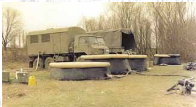
Figure 88. Water station for complex water purification
