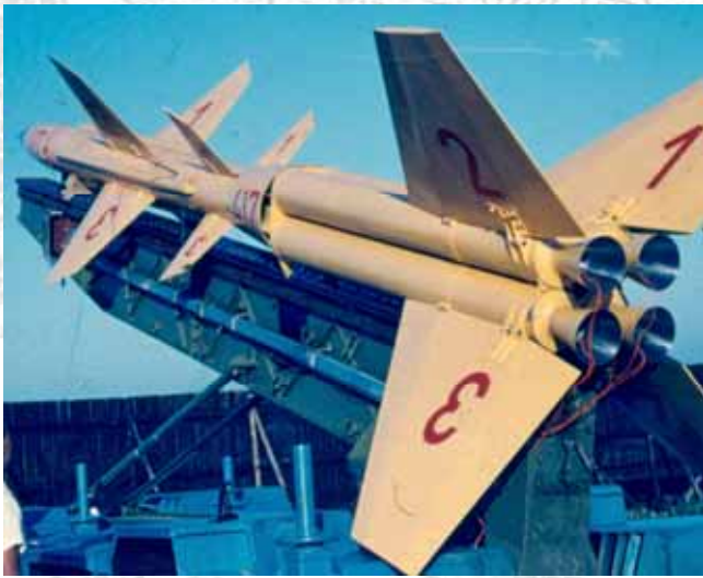
Figure 23. The two-stage ground-to-air missile VULKAN
