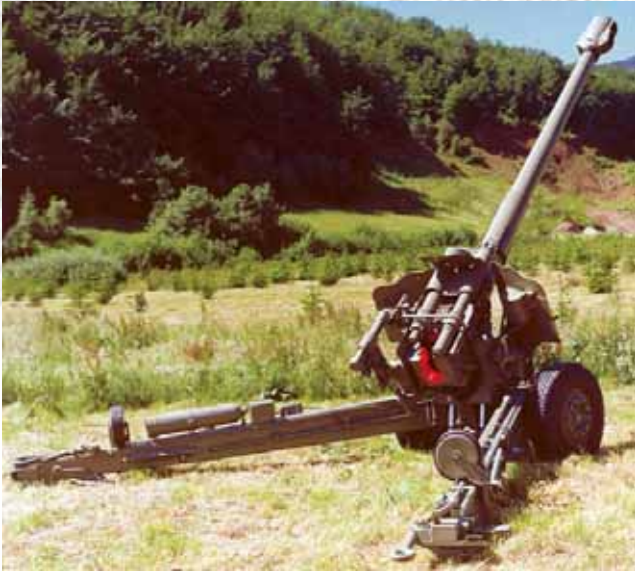
Figure 11. Gun-howitzer 152 mm NORA-A (M-84) version with projectile thrust
