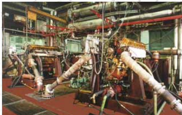
Figure 98. Engine test stand with 1900 kW power rate
