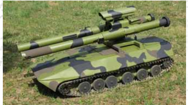
Figure 36. Mobile modular robotized anti armour system MILICA
