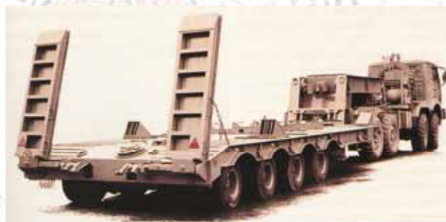
Figure 54. Towed vehicle FAP 3232 with a low-carrying semi-trailer with a capacity of 45 t
