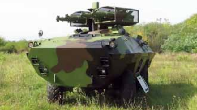
Figure 34. Armored combat vehicle BOV-3 armed with MALJUTKA 2T5 missiles
