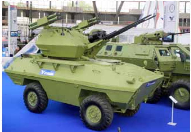
Figure 18. 20/3mm self-propelled anti-aircraft gun BOV-3 with rocket launchers STRELA-2M
