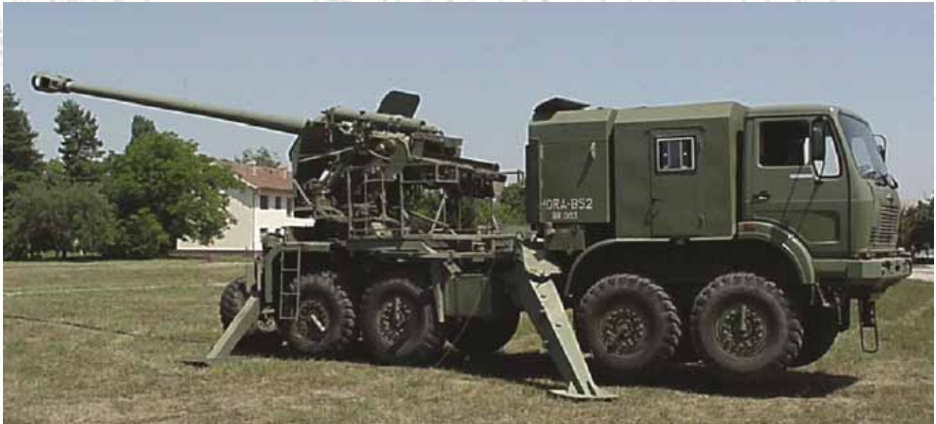
Figure 12. Self-propelled 155 mm gun-howitzer NORA-B52
