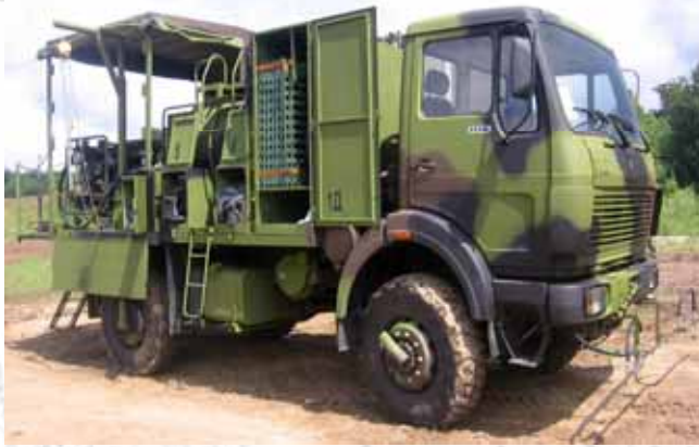
Figure 83. Special CBRN vehicle with the SANIJET S.921 decontamination device
