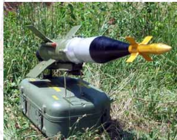
Figure 32. Antitank launching kit MALJUTKA-2T with the tandem warhead
