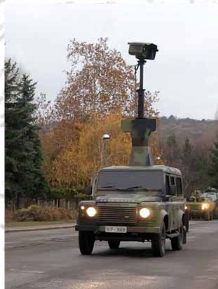
Figure 78. MIP-11 multi-sensor intelligent platform
