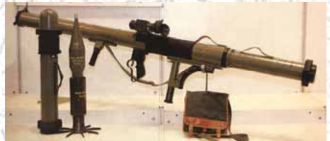
Figure 31. 90 mm portable rocket launcher M79 OSA
