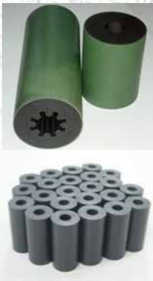
Figure 95. Propellant NGR-316 of flight rocket engine of the BUMBAR system
