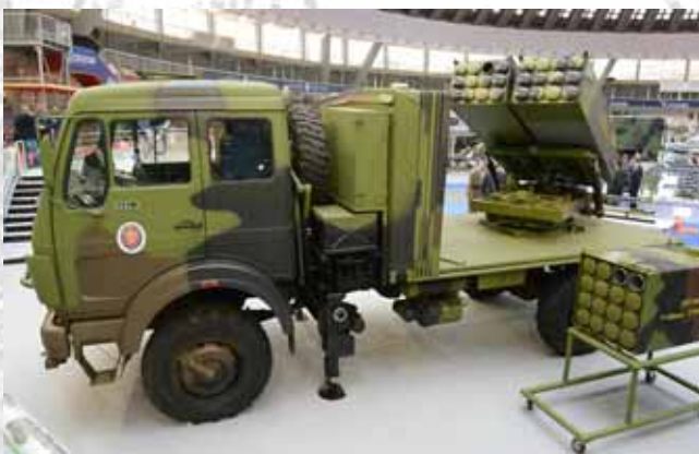
Figure 30. Modular multi-launch self-propelled rocket system LRSVM (MORAVA)
