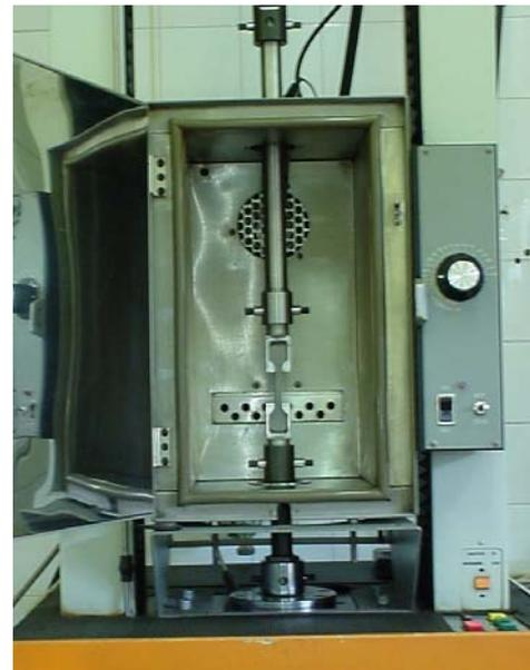
Figure 7. Universal tester for tensile measurements
