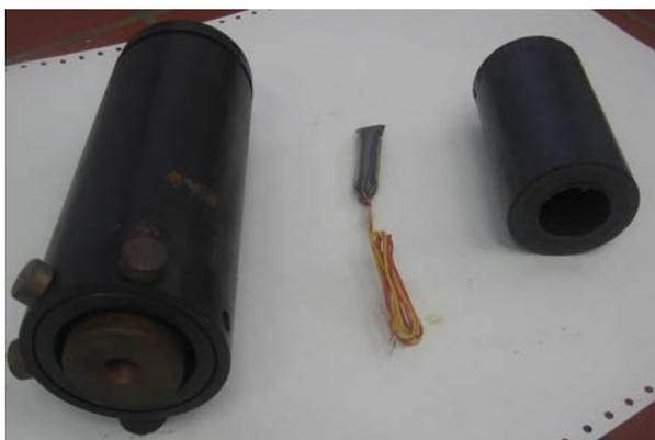
Figure 9. Two inch motor: grain, igniter and metal parts
