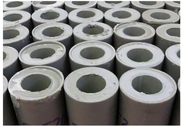
Figure 6. Cast grains for 2 inch motors
