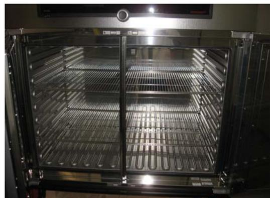
Figure 8. Temperature chamber for curing propellants
