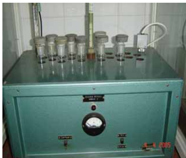
Figure 1. Artificially ageing of NC-40 MBL 9226
