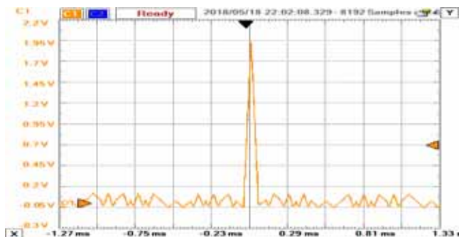
Figure 6. The autocorrelation of binary phase sequence obtained using the FPGA Zedboard
