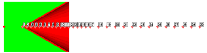
Figure 6. Gauges position used to measure the axial velocity of the jet
