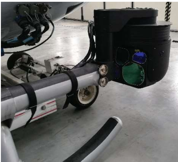
Figure 11. Thermal imaging camera on EC 135 in pre-flight position
