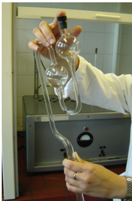
Figure 2. Replacing the solvents into the heating tube after heated at 132 °C for 5 hours
