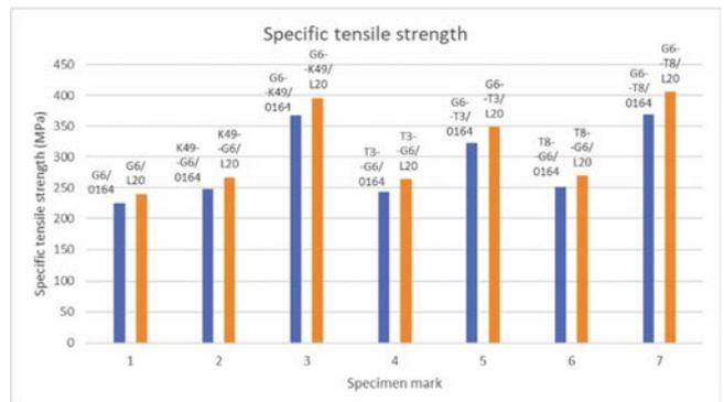
Figure 12. Specific tensile strength of two single fiber and twelve hybrid filament wound composite materials versus epoxies 0164 and L20
