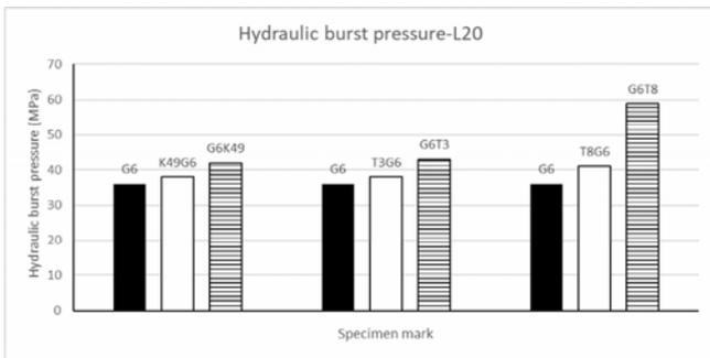
Figure 8. Hydraulic burst pressure of single fiber tubes and hybrid tubes with epoxy L20
