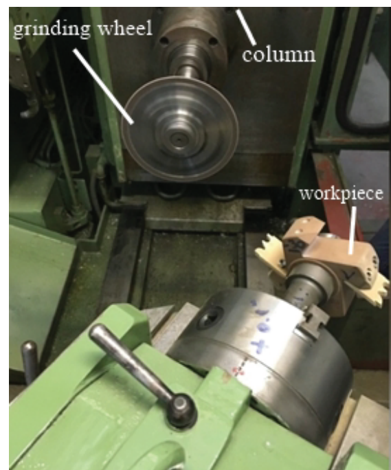
Figure 3. 3+2-axis grinding operation on a horizontal machining center
