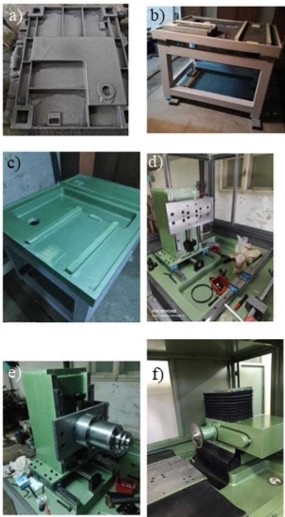
Figure 7. Steps of building 3+2-axis CNC machine – Profiator 100
