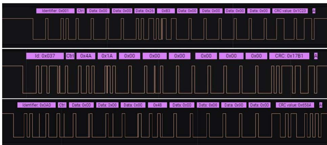
Figure 13. Data frames from the connected nodes on the CAN bus
