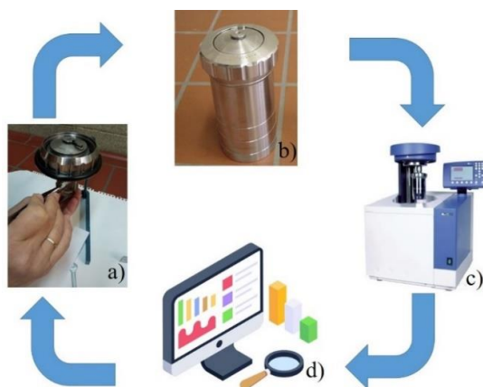
Figure 6. Analyzing the sample a) Positioning the sample in a quartz container, b) Introducing inert gas, c) Conducting the experiment in the calorimeter, d) Analyzing the acquired results
