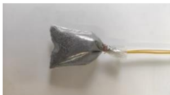
Figure 1. Prepared sample of a pyrotechnic mixture in polyethylene bag
