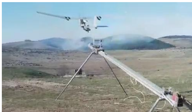
Figure 8. Sparrow UAV catapult launch
