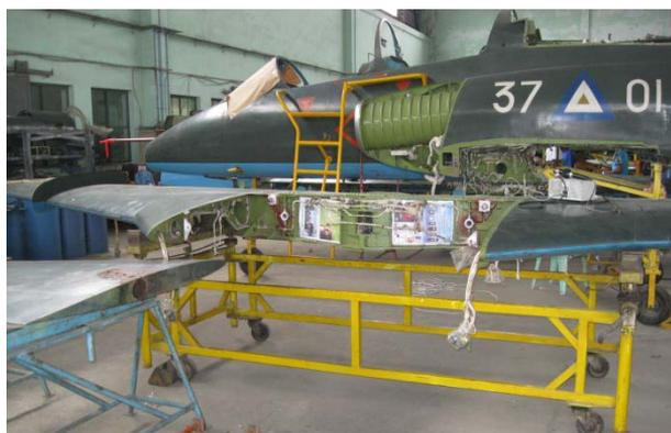
**Fig. 2.** Structure of aircraft Super Galeb G-4
