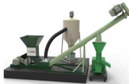
Continuous pellet production unit
