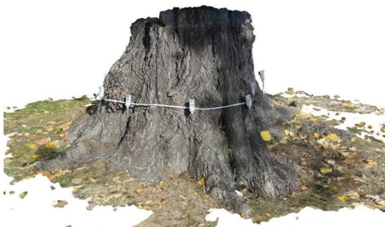
Figure 7. Photogrammetric 3D model of tree trunk
