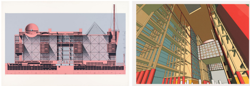
FIGURE 5: Final screen-printed and longitudinal section view of the proposal for New Tokyo City Hall, with colour separation indicating an understanding of layering procedures common to contemporaneous CAD software, and potentially themselves produced from computer generated models captured in additional in-process perspectives, produced by consultant firm ARC Yamigawa using the McDonnell Douglas-produced Graphic Design System with additional development by Applied Research of Cambridge (ARC); Left: Longitudinal Section of Main Building for the Tokyo City Hall Competition Entry. Printed 1986. Screen Print. 58,2 x 115.0 cm. DR1988.0274. Canadian Centre for Architecture. © Arata Isozaki; Right: View of Atrium, looking up for Tokyo City Hall Competition Entry. 1986. Computer-Aided Design Print. 76.8 x 108.6 cm. DR1988.0273. Canadian Centre for Architecture. © Arata Isozaki.
