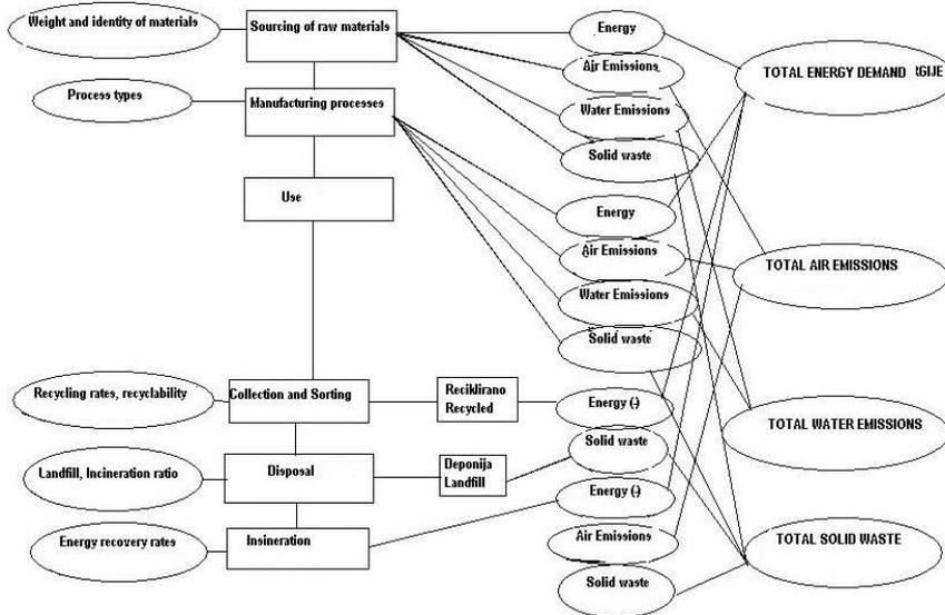
Fig. 2. A schematic showing the working of the lifecycle model
