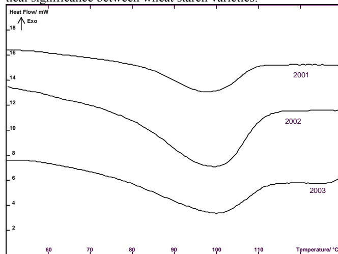
Fig. 1. Thermograms of dissociation of AML from starch of Symfonia variety harvested in 2001-2003
