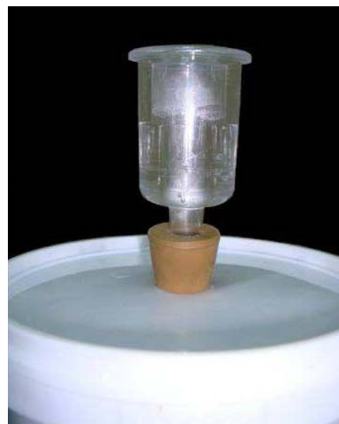
Fig. 2. Cover of the container with rubber seal and water-valve
