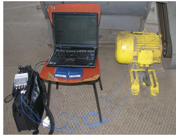
Fig. 4. Instrumentation for vibration signal acquisition and fault detection
