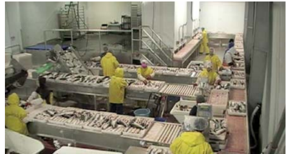
Fig. 4. Panning and weighing sub-system
