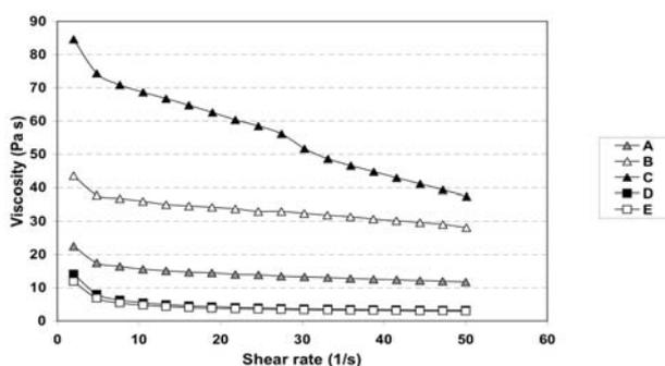
Fig. 2. Changes of viscosity (Pa s) of dark chocolate samples, during mixing (A), pre-refining (B), refining (C), conching (D) and tempering (E) steps
