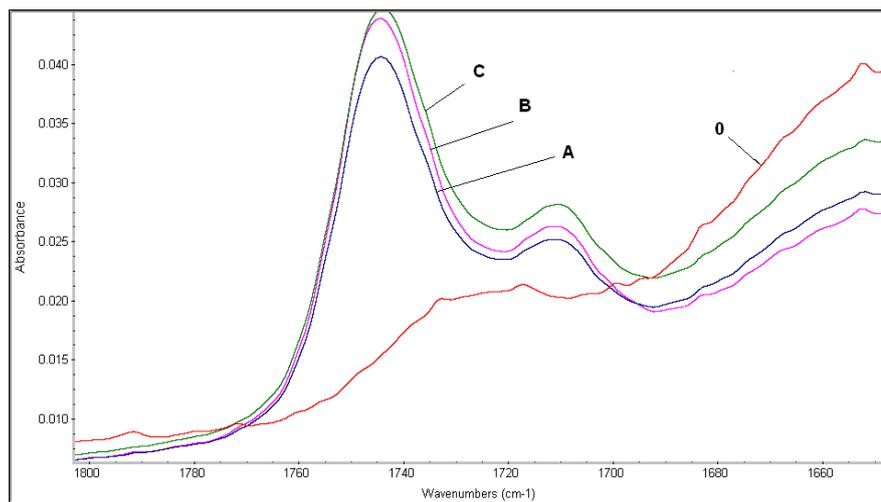
Fig. 3. Essential oil interactions in spectral region 1650 -1800  $\text{cm}^{-1}$ : 0 – blank shot film, A – 0.5% oil, B – 1% oil, C – 2% oil
