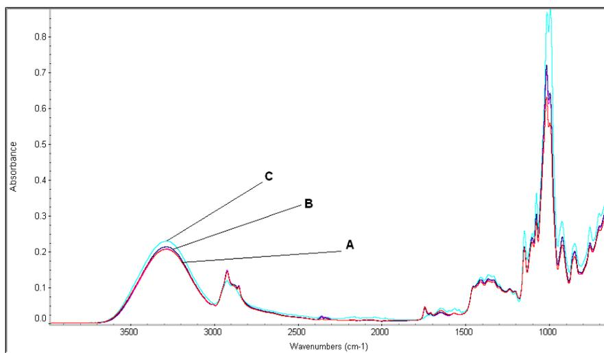
Fig. 2. FTIR spectra of samples with different oil concentration: A – 0.5% oil, B – 1% oil, C – 2% oil
