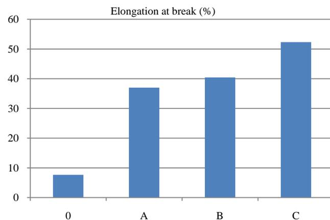
Fig. 1b. Elongation at break of films with different oil concentration (%): 0 – blank shot film, A – 0.5% oil, B – 1% oil, C – 2% oil
