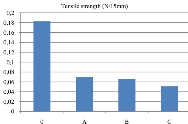
Fig. 1a. Tensile strength of films with different oil concentration (N/15mm): 0 – blank shot film, A – 0.5% oil, B – 1% oil, C – 2% oil
