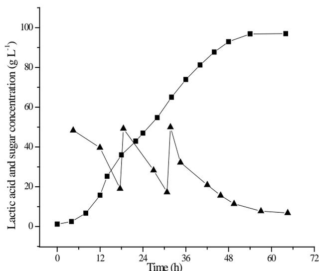
Fig. 2. Fed-batch lactic acid fermentation on complete stillage. Symbols: square - lactic acid concentration ( $\text{g L}^{-1}$ ), triangle - sugar concentration ( $\text{g L}^{-1}$ )
