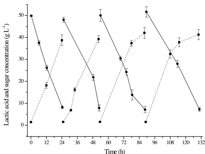
Fig. 3. Lactic acid fermentation on liquid distillery stillage by immobilized cells of *L. rhamnosus* ATCC 7469. Symbols: dot lines - lactic acid concentration ( $\text{g L}^{-1}$ ), solid lines – sugar concentration ( $\text{g L}^{-1}$ )
