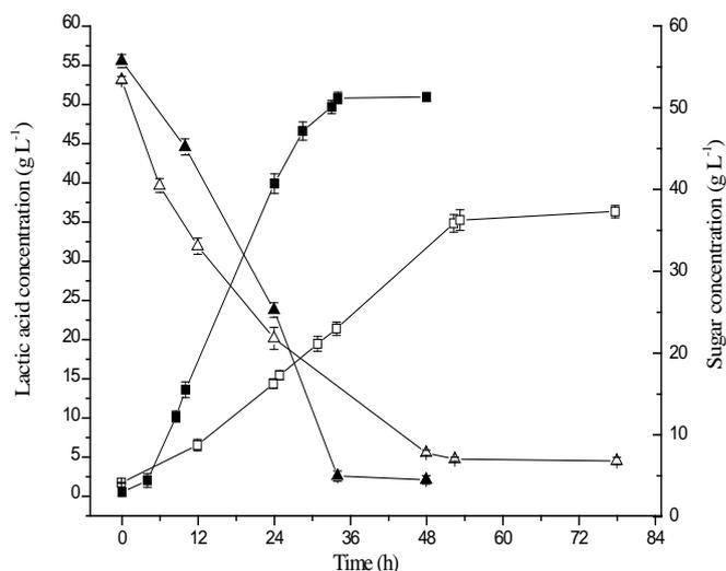
Fig. 1. Kinetics of batch lactic acid fermentation on complete stillage and liquid stillage. Symbols: square - lactic acid concentration ( $\text{g L}^{-1}$ ), triangle - sugar concentration ( $\text{g L}^{-1}$ ), solid symbols - whole stillage, open symbols - liquid stillage
